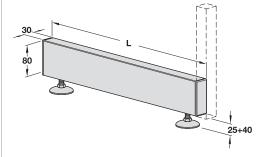
> Area of application: Foot for columns 30 x 30 mm and  $60 \times 30$  mm
