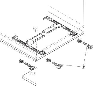
Hinge carrier strip set 2 Flap fixing set
