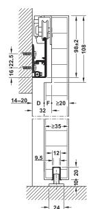
Clear threshold floor guide, with guide track
