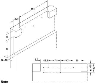
Predefined screw positions simplify the installation. We recommend pilot drilling the drilling pattern when recessing the cut-out.
