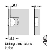
Application and planning dimensions for base panel thickness
