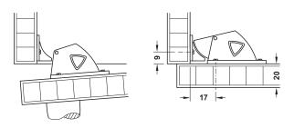
The latchbolt is retracted and the door can be opened when presenting the whatlock® magnetic key (not supplied). The latchbolt engages automatically when the door is being closed. The door is secured.
