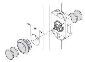
For Push-Lock locks operated from one side the following are required: 1 push-button and 1 rosette (for locks operated from both sides: Additional push-button)
