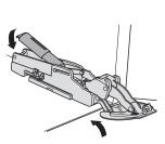
Clip soft opening mechanism into rear axle
