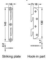
> Mounting: For right and left hand use Striking plate for recess installation and screw fixing, hook-in part for screw fixing Installation:
