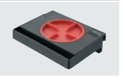
For floating installation of laminate and prefinished parquet floors without wedges, continuously adjustable for wall distance 5-20 mm, with practical turn knob, wide clamping and support surface, with millimetre scale, robust, light and compact Material: plastic
