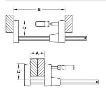
For clamping and spreading of sensitive surfaces, round and sharp workpieces with large clamping surfaces, also tightens on the side and behind the rail, clamping force up to 1,500 N  $\,$
