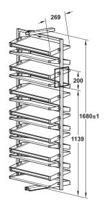
Version: Pull out shoe rack rotates through 180°
