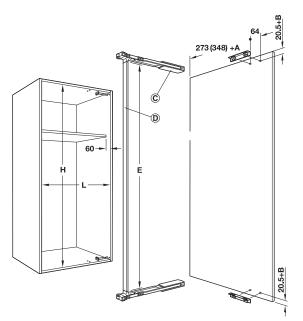
C Door opening mechanism, D Connecting bar
