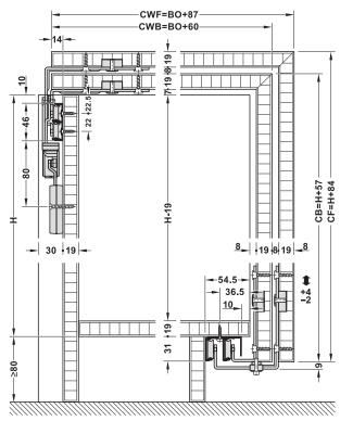
H = height BO = base panel depth CF = front door height CB = rear door height CWF = front door depth CWB = rear door depth
