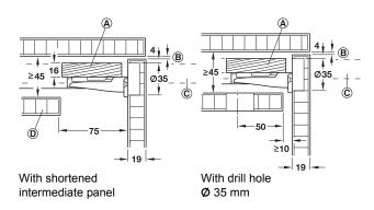
(A) Wooden strut (B) Gap (C) Door (D) Intermediate panel
